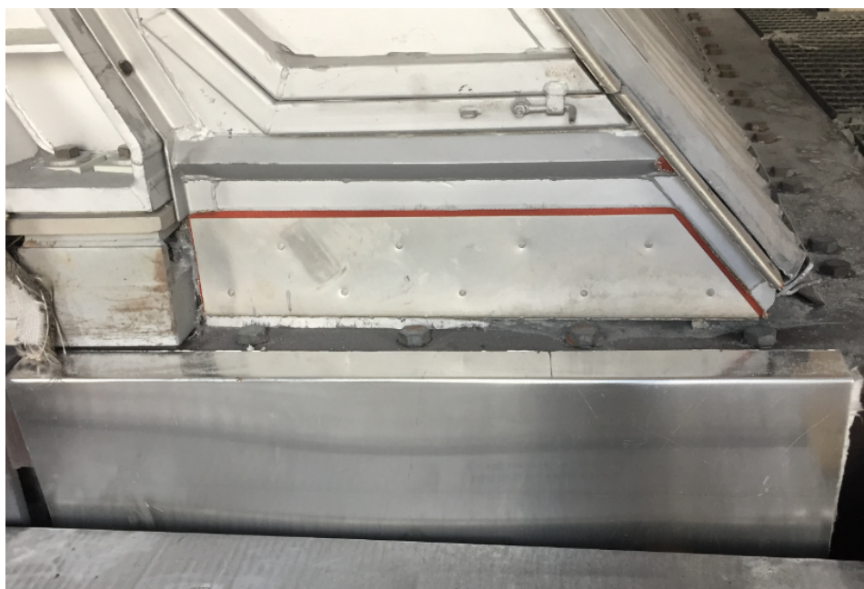
Figure 7. Heat deflectors used to increase side- and end-wall insulation of D20+ cell.
